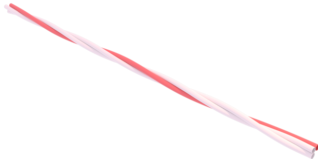
Figure 2: Example of three fiber twisting with line-to-line contact.
